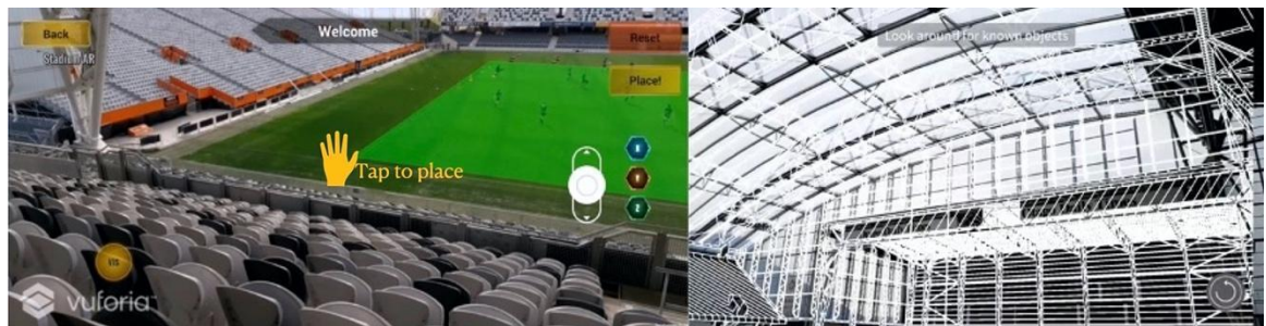
Figure 2: Localization methods for AR interface. Left) User-guided localization requiring the user to input seat location and provide alignment to a digital pitch map. Right) Automatic model-based localization using a 3D model of the stadium.
