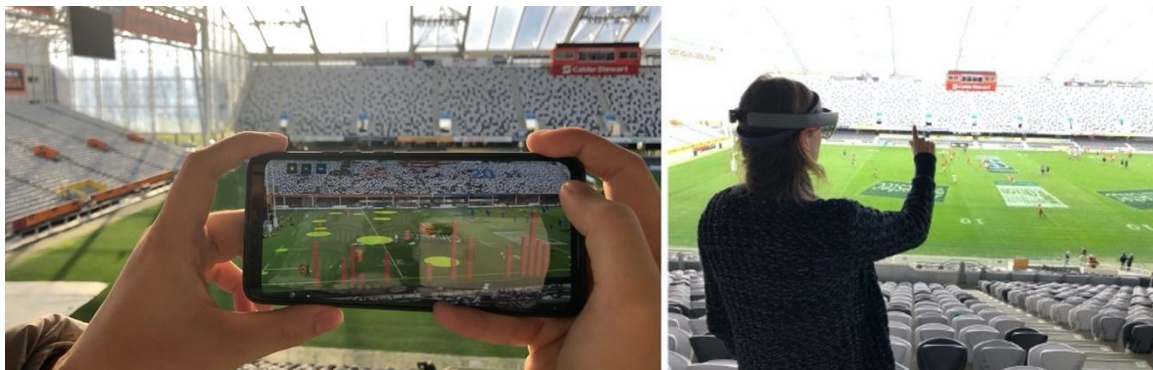
Figure 1 AR interfaces for sports spectating. Left) AR interface on mobile phone using video-see-through AR. Right) User with optical-see-through AR interface (HoloLens) used for sports spectating.
