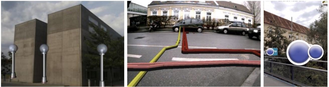
**Fig. 3:** Visualization problems caused by naïve compositing functions. Left) Virtual planned lamps are perceived to be located in front of the house not next to it. Middle) Virtual pipes seem to float above the ground. Right) In this tourist scenario the naïve overlay of sight labels produces information clutter.
