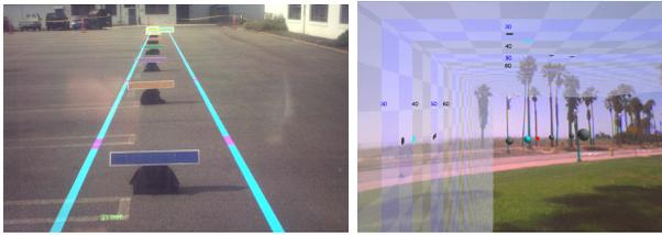
**Fig. 11:** Examples for using external virtual cues. Left) Adding a set of parallel lines to improve the depth perception (Image courtesy of the U. S. Naval Research Laboratory, Livingston et al. [35] ©[2009] IEEE). Right) Virtual Shadow Planes for visualizing absolute depths (Wither et al. [63] ©[2005] IEEE).
