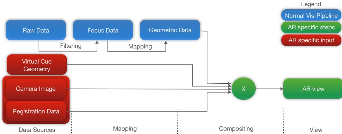
**Fig. 10:** Pipeline for creating external virtual cues. An external geometry is added to the compositing step in order to create additional depth cues. The camera image is only needed for video see-through displays or when extracting other image features.
