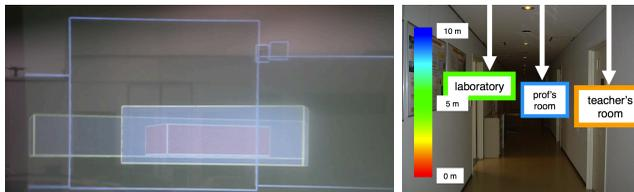
**Fig. 13:** Mapping from distance to appearance. Left) Using intensity and opacity for encoding depth (image courtesy of the U. S. Naval Research Laboratory, Livingston et al. [112] ©[2003] IEEE). Right) Using color to encode distance (Uratani et al. [62], ©[2005] IEEE).
