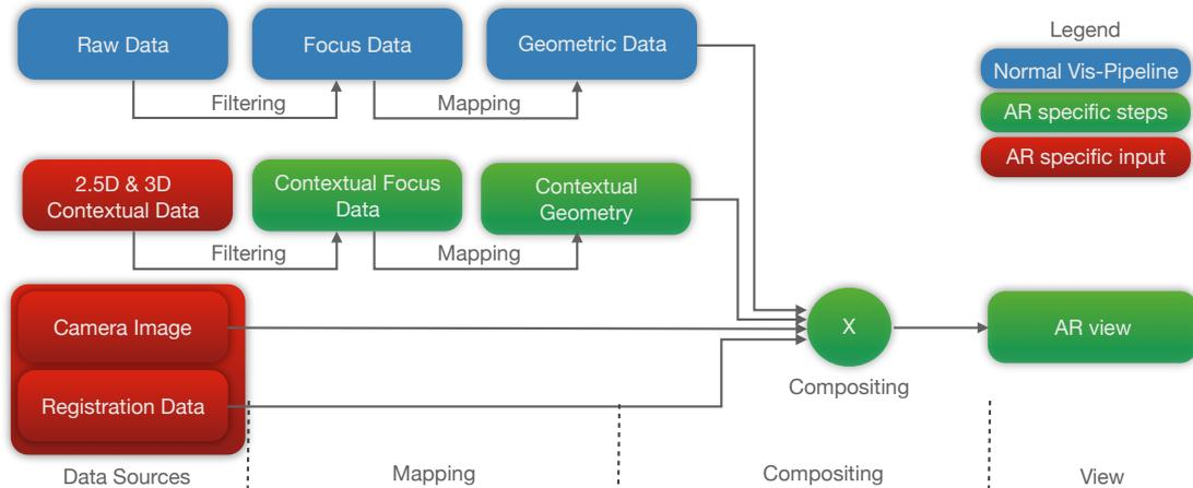
**Fig. 8:** Pipeline for creating model-based physical cues. A 2.5D or 3D representation of the physical world is used as additional input for the visualization to create physical cues. The camera image is only needed for video see-through displays or when extracting other image features.
