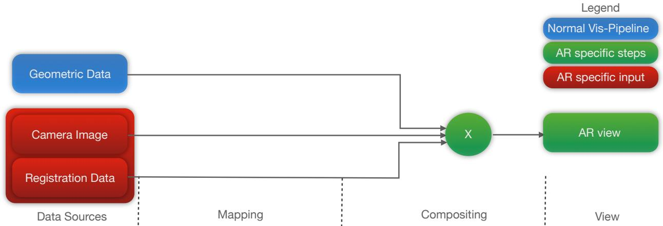
**Fig. 2:** AR Visualization Pipeline illustrating a naïve overlay using predefined geometric data, a camera image and registration data for creating the compositing.
