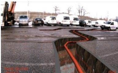
**Fig. 15:** Cutaways as virtual cues in AR. A virtual excavation with a depth scale is used to visualize subsurface infrastructure (Zollmann et al. [113]).
