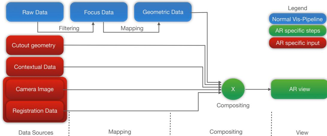
**Fig. 14:** Creating additional virtual cues with cutaway geometries. The camera image is only needed for video see-through displays or when extracting other image features.
