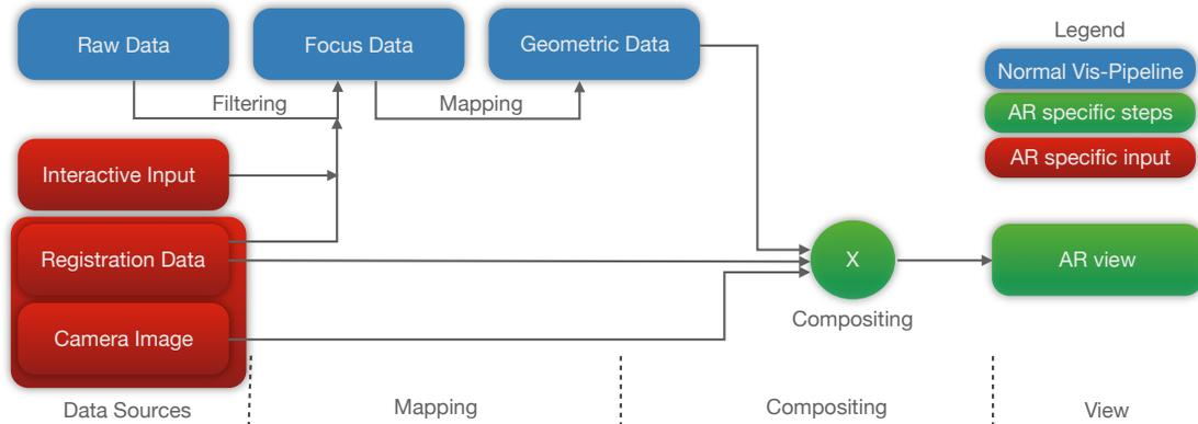
**Fig. 16:** Information filtering pipeline. The camera image is only needed for video see-through displays or when extracting other image features.
