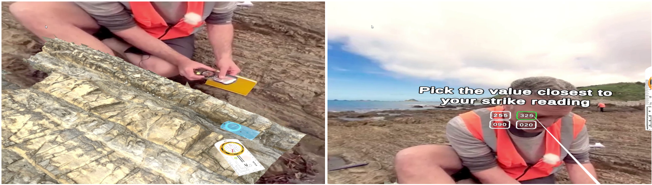
Figure 3: (Left): Students are shown the correct position to place their compass in in order to measure the strike of a virtual bedding plane. (Right): The student is presented with a multichoice question asking the strike of the virtual bedding plane.
