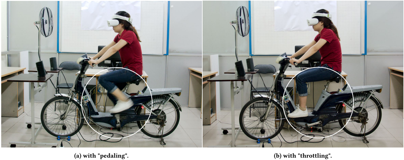
Figure 3: A participant was performing the experiment. She had to use her legs to pedal the bike (on the left). In contrast, the movement was indirectly powered when she throttle by using her right hand (on the right).
