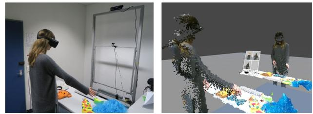
Figure 3: Left: User interacting with real objects in voxel space; Right: Virtual third person view of the mixed scene.
