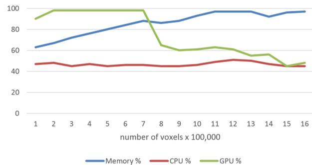
Figure 13: System behaviour under increasing voxel number load; i7 6700, 3.4 GHz, 16GB RAM, GTX970, 4GB
