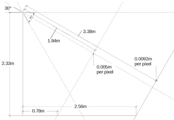
Figure 4: Resolution of Kinect depth data in relation to distance from sensor.
