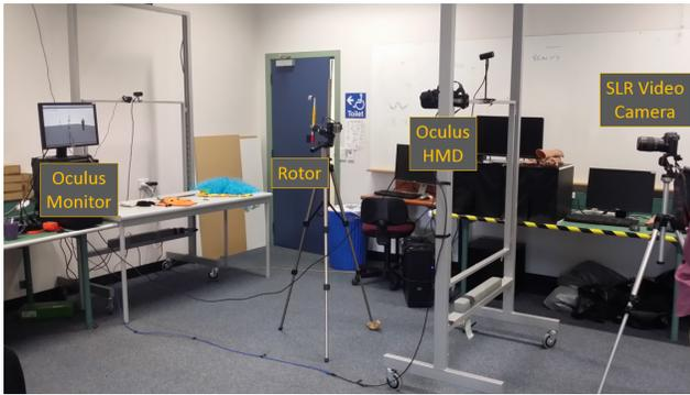
Figure 10: Setup of latency measurement: SLR Video Camera is capturing the Oculus Monitor *and* the Rotor; the Oculus Monitor presents what is seen by the Oculus HMD looking at the Rotor.
