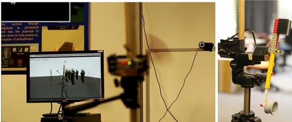
Figure 11: Left: Example frame taken from video stream recorded by SLR Video Camera showing both the Oculus Monitor and the Rotor in action; Right: Photo of the Rotor build for the latency measurement rotating with about 360 revs/min.
