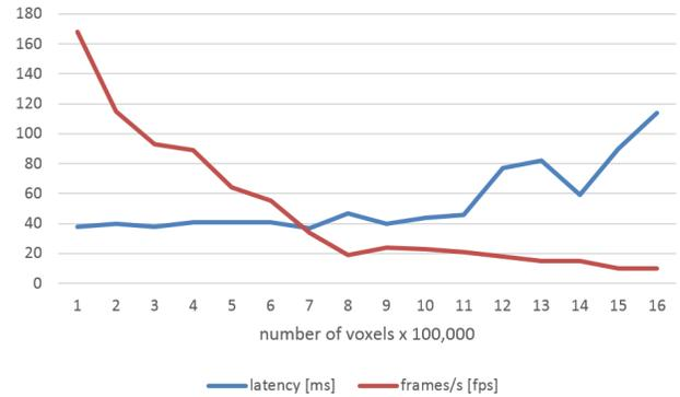
Figure 12: Framerate and latency developing with increasing numbers of voxels present in scene; measured at 100,000 voxels intervals.
