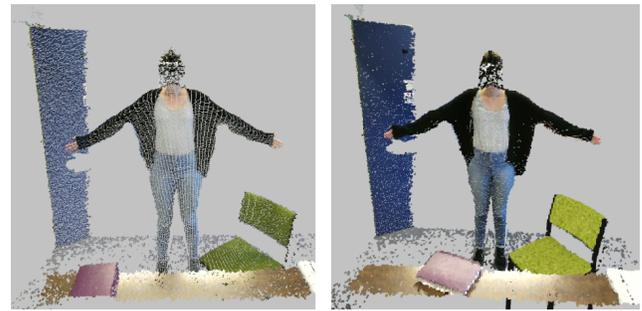
Figure 5: Visual effect of different voxel sizes at interaction distance: Left: voxel size = 0.5cm, Right: voxel size = 0.8cm. Increasing voxel resolution does not necessarily leads to better visual quality.
