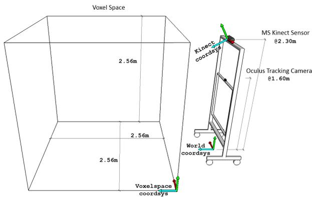
Figure 2: General setup of Mixed Voxel Reality system: The user interacts within a  $2.56^3 \text{ m}^3$  space in front of a Kinect camera while wearing a head-mounted display tracked by a camera in front of him/her.
