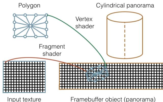
Fig. 3. Mapping the panorama on the GPU to achieve real-time generation and update of the panorama on mobile phones. The panorama is stored in a framebuffer object. For each incoming camera frame a vertex shader maps a polygon into the panorama space based on the transformation gained from visual tracking. In a second stage a fragment shader reads back colours from the input texture (the camera image) to the panorama.
