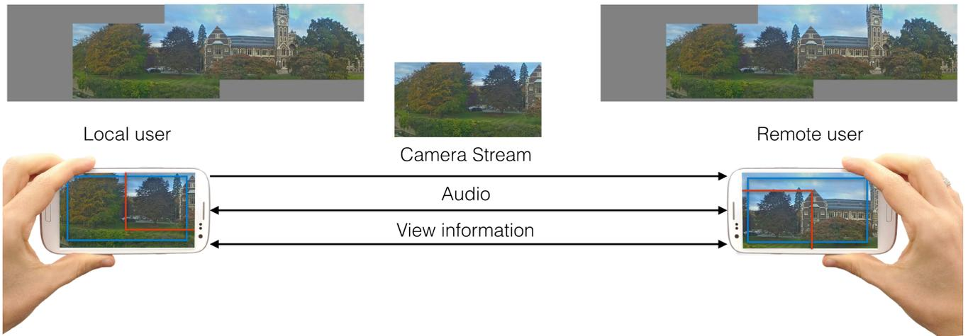
Fig. 2. Overview on our PanoVC system. The local user creates a panoramic image from the camera stream which is also used for vision-based tracking. The camera stream is sent to the remote user where it is used to create and update a panoramic image of the distant environment. Additionally, the user exchange audio and view information. View information allows both users to see where they are currently looking.
