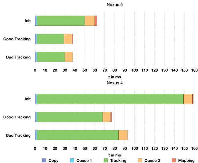
Fig. 6. Average timings for updating the panorama during different stages. For each device we measured the average time to process an incoming camera frame for the first 10 frames (init), a steady movement with panorama generation (good) and a jerky movement with bad tracking results where the tracking fails (bad). In the latter case no mapping is performed.
