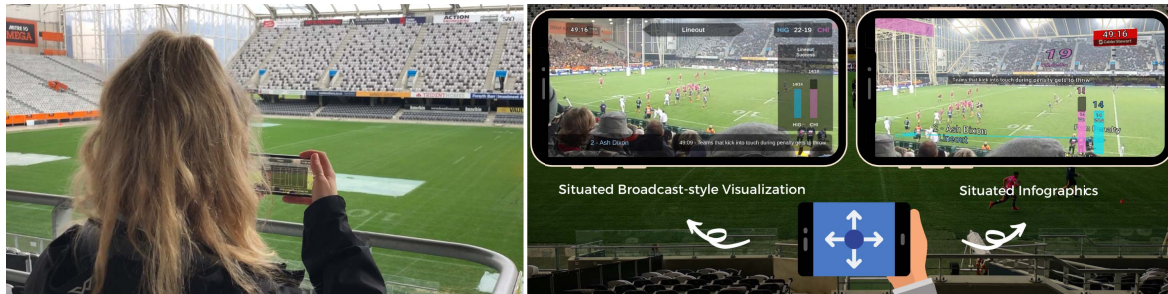
Figure 1: On-site situated visualization for sports spectators. Left) Our prototype used in the real stadium environment. Right) Illustrated user's view of situated broadcast visualization (left) with graphics in screen space and situated infographics visualization (right) with graphical elements embedded spatially into the stadium environment.
