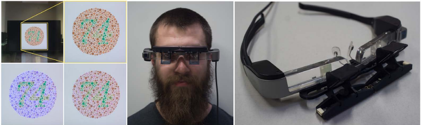
Figure 1. ChromaGlasses overview: (Left Top) Standard Ishihara test marker as seen through non-active glasses and cropped region. People suffering from red-green colour vision deficiency tend to see "21" instead of the correct "74". (Left Bottom) The same test marker when seen through active ChromaGlasses. A pixel-precise overlay causes a shift revealing the correct "74". However, depending on the severity, a less drastic shift might be sufficient. (Middle and Right) ChromaGlasses prototype for creating a precise correction overlay utilizing current optical-see through head-mounted displays extended by custom cameras demonstrating possible miniaturization.
