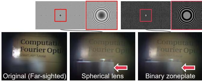
Fig. 9. Diffraction lens demonstration. A viewpoint camera focuses at a far object. We display a spherical lens phase pattern and a binary zone plate pattern of the same focal length separately. The resulting images in the bottom center and in the bottom right both focus on a near object. Note that the binary intensities of the zone plate image so that their retardation is a half of the base wavelength.
