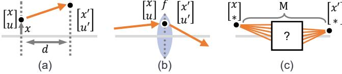
Fig. 4. Ray transfer matrix analysis. (a) A ray transfers space. (b) A ray transfers a thin lens. (c) Two points that are conjugate each other for a given ray transfer matrix.
