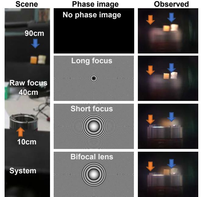
Fig. 10. Bi-focus mode. (left) The scene. The camera focus is set at around 40cm from the system. We located other objects at 10cm and 90 cm respectively. (center) Phase images. The bottom image is a bifocal lens image that renders a concave lens in the inner area and a convex lens in the outer area. (right) The bifocal lens allows the camera to focus on both objects simultaneously.
