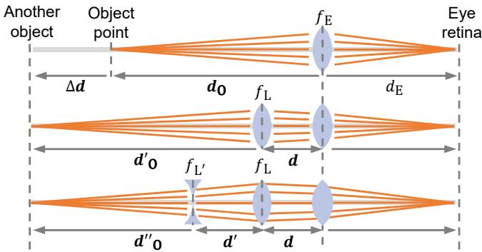
Fig. 6. Schematic diagram for the explanation of the lens simulation in Sec. 3. Note that the focal length of the additional lens,  $f_L$ , usually takes a negative value, so the lens becomes a concave lens. In this figure, however, we draw it as a convex lens for the readability of the figure, and switching the sign of  $f_L$  does not affect the derivation of  $f_E$ .
