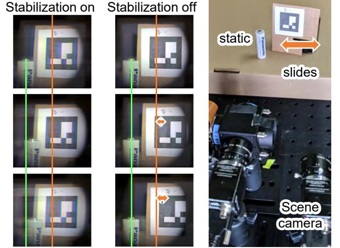
Fig. 13. View stabilization along the x (horizontal) axis controlled by placement of a fiducial marker. The view shift is set to the displacement of the marker's initial X position. (left) Stabilization is on. (center) Stabilization is off. (right) Application setup. The red and green lines are for guidance only.
