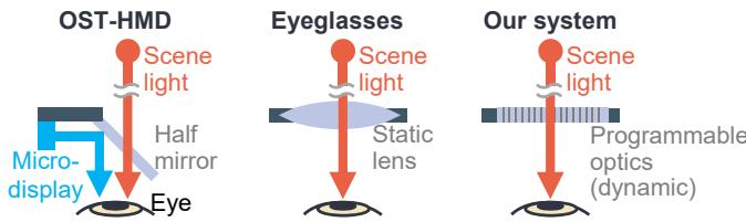
Fig. 3. General overview of traditional eyewear and our approach. (left) A typical OST-HMD optics. (middle) Eyeglasses. (right) Conceptual optics design of our approach.
