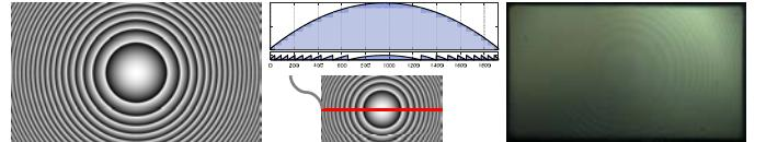
Fig. 2. A PSLM can display a computational lens. (left) An input spherical phase pattern. (middle) The intersection of the pattern. The pattern is a Fresnel lens of a convex lens. (right) An actual lens image captured while focusing at the surface of the PSLM. The phase pattern behaves as if there is a thin lens layer on the PSLM.
