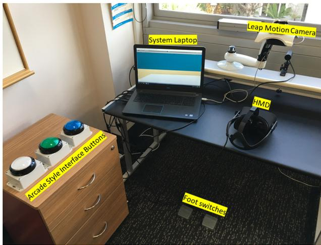
Figure 3: Demonstration of the Home Rehabilitation System setup which includes: three “arcade” style buttons (left) to operate the different system modules, two foot switches (under table) to interact in system while wearing HMD, and a desk with wheels that can easily moved around a patient’s home.
