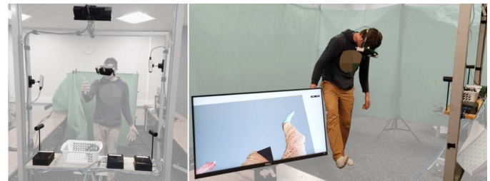
Fig. 1. A real-time reconstruction system for embodied experiences, using two stationary exocentric stereo cameras in combination with two egocentric stereo cameras attached to an HMD (left). The first-person view of the user shows a dynamically reconstructed virtual body with data contributed from both the exocentric and egocentric cameras (right).
