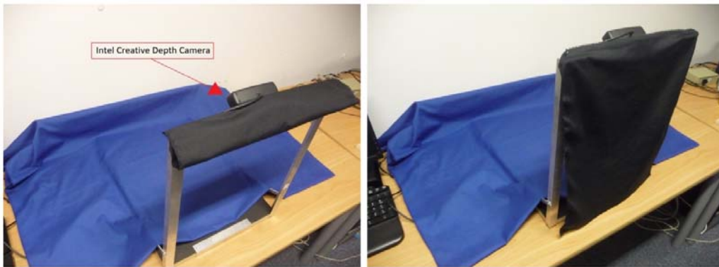
Figure 2. Metal Frame used to position the depth cam without curtain (left) and with the curtain to prevent the direct view of the hand during use (right)
