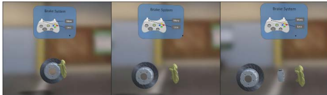
Figure 5: The figures above demonstrate the virtual brake assembly (left) with an accompanying display presenting the assembly name and a picture of the interaction device (XBOX controller) identifying possible controls. The brake assembly can be separated into its main components (middle and right).
