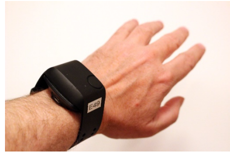
Figure 8: Empatica E4 wristband to measure electro-dermal activity heart rate, acceleration, and skin temperature before, during, and after VR exposure. Unfortunately, it is very difficult to get reliable data in non-laboratory conditions.
