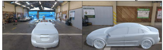
Figure 3: The figures above demonstrate the virtual car inserted into the environment surrounded by the panoramic workshop. Each figure is taken from a different position in the workshop. A basic model car is used as a placeholder for demonstration purposes. We perform shadow rendering onto an invisible plane to achieve visual coherence of the scene and provide depth cues.
