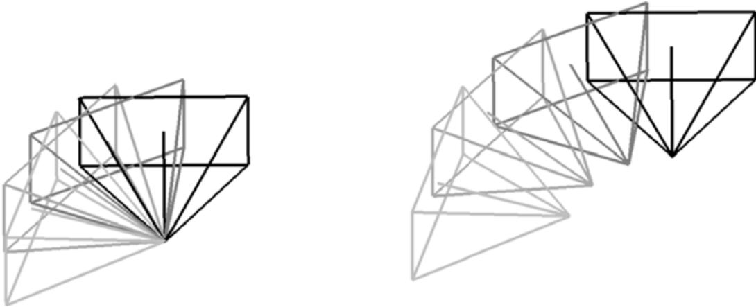
**Figure 1.1** Pure rotation trajectory (left) containing no translational movement, compared to a more realistic spherical movement (right).
