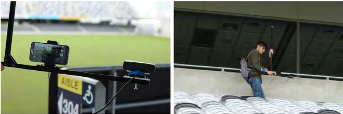
**Figure 3.6** The complete stereo-rig being used to capture in the stadium. Left: close-up of the view from the stereo-rig. Right: how the rig was held, including the backpack setup.
