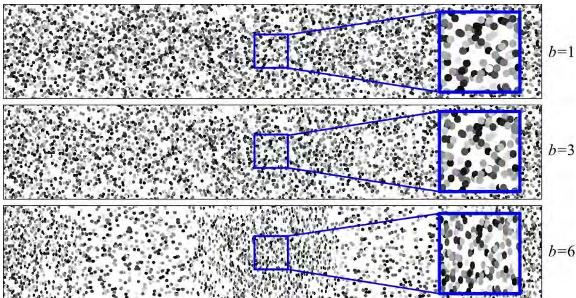
**Figure 6.8** Synthetic panoramas produced by spherical tracking of elliptical movement through random points. With  $b = 1$ , the camera moves in a perfect circle, resulting in an even distribution of points. Our system could generate panoramas with large elliptical deviations; however, the originally circular points become distorted with the large values depicted with  $b = 3$  and  $b = 6$ .
