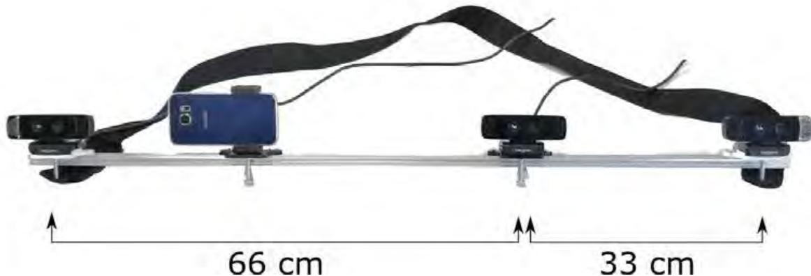
**Figure 3.5** Diagram of the stereo rig with four cameras. Three cameras are calibrated before and after the capture session, with three main baseline configurations (33 cm, 66 cm, and 1 m). The mobile device camera is also calibrated to allow for comparisons with the other cameras, which may be used as a baseline or ground-truth.
