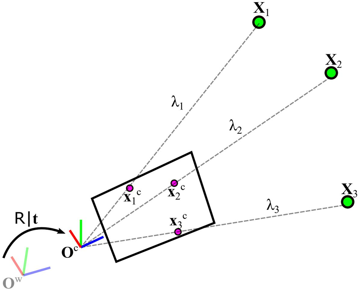
**Figure 2.1** Depiction of the Perspective-3-Point (P3P) problem. A camera centred at  $O^c$  observes projections  $x_i^c$  of corresponding 3-D points  $X_i$ . The objective of the P3P problem is to find the camera pose  $[R | t]$  that supports those correspondences.
