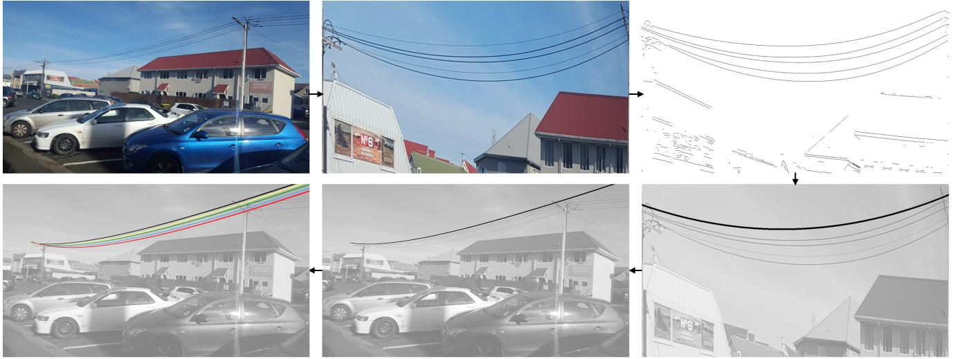
Fig. 2. Example of our method for power line detection. Clockwise from top-left: Input image, perspective transformation is applied, image is filtered, power lines are detected, reverse perspective transformation is applied to the wires, separate lines can be distinguished in the original image.
