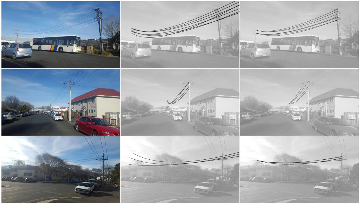
Fig. 5. Comparing the line tracer to the randomized Hough transform in three cases. From left to right: input image, line tracer output, randomized Hough transform output.
