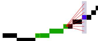
Fig. 4. One iteration of the line tracing algorithm. The green pixels represent pixels traced in previous iterations. The red lines indicate the candidate segments. The blue pixel is the predicted end-point.
