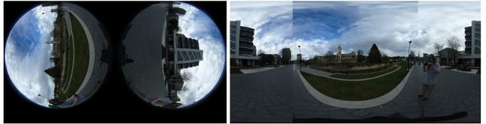
Fig. 8. An example of the 360° images we obtain from the Ricoh camera. (Left): The raw dual-fisheye image provided by the camera. (Right): The result of projecting this image into our equirectangular panorama.
