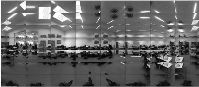
Fig. 7. A pre-captured environment split and unprojected into multiple segments for feature matching. The relative rotation between new camera frames and the segment with the most matches to the new frame is combined with that segment's rotation to calculate the absolute orientation of the user's device.
