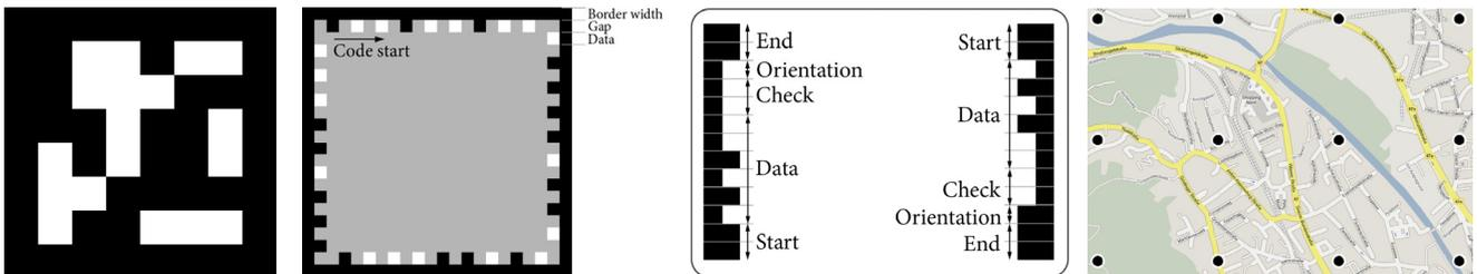
Figure 1. Left: regular black/white marker, 2<sup>nd</sup> to 4<sup>th</sup> images: layout of frame markers, split markers and dot markers.
