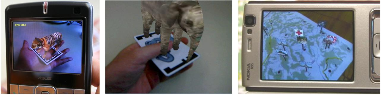
Figure 4. frame markers (left), split markers (middle) and dot markers (right) used on mobile phones.
