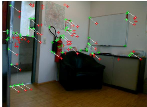
Figure 7. Flow vectors from feature matching.
