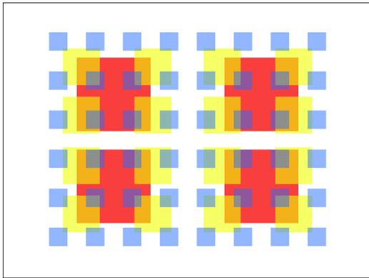
Figure 8. Areas for region-based matching. In the first iteration, the 4 large red areas, then the 16 yellow and finally the 48 blue areas are matched.
