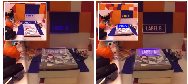
Figure 1: Eye-perspective rendering provides AR applications with information about the user's view of the scene by synthesizing their view through an optical see-through display. (Left) Using input from a built-in head-mounted display camera that films the real-world scene (small inset image), a view management algorithm places labels suitable for the respective background areas. Due to the viewpoint offset between camera and the user's eyes, the user actually perceives the label in a different location causing a lack of contrast. (Right) Eye-perspective rendering synthesizes the user's view through the display (small inset view) that is then used by view management algorithms to adapt labels in order to avoid visual interference with the background.
