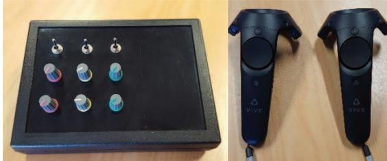
Figure 2: Our version of Arnold's six-dial device for manipulation of the Hypercube (left) and HTC Vive controllers used for the immersive VR condition (right).
